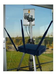
The "wireless mesh" is an ad-hoc and mobile network based on Wi-Fi technology. Each MRX station serves as relay point as well as access point within the mesh. The mesh can be arbitrarily enlarged and designed redundantly. New MRX stations are automatically recognized and integrated into the mesh. All user data and communication within the mesh are encrypted. Only devices that know the mesh-key can log in, collaborate and send/receive data.
