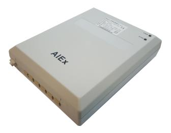
The AIEx (Alarm Extender) device is a telecontrol system that transmits local alarm signals via its G.703 64kbit/s interface to a remote alarm controller unit, which outputs the alarm via relay contacts. It enables to manage and supervise alarm systems, fire detection systems or similar devices via parallel I/O ports.
